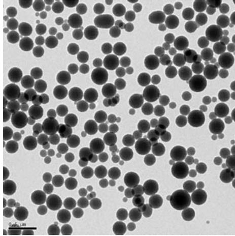
*Figure 5. TEM image of  $\alpha$ -lactalbumin nanoparticles in the examined sample (courtesy of Nia Bell of UCSD). The images were acquired with a FEI Tecnai G2 Sphera at 200 KV. The scale bar in the lower left corner of the image corresponds to 500 nm.*
