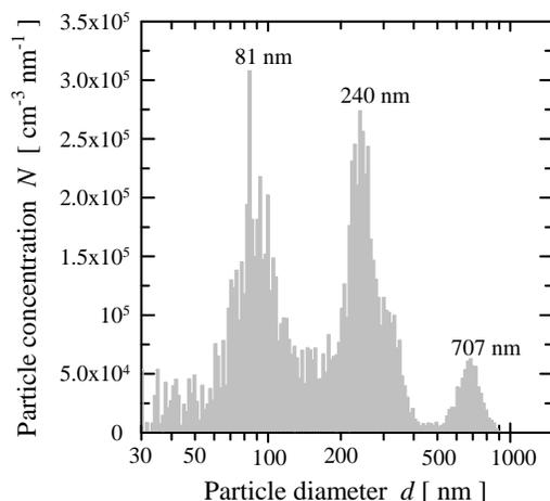
Figure 3. As in Figure 1 but the results were obtained for a polydisperse sample consisting of the mix of three polystyrene nanosphere size standards, 81 nm, 240 nm, and 707 nm. The concentration of particles integrated between 0 and 1,000 nm for this sample was about  $5.0 \times 10^7 \text{ cm}^{-3}$ .
