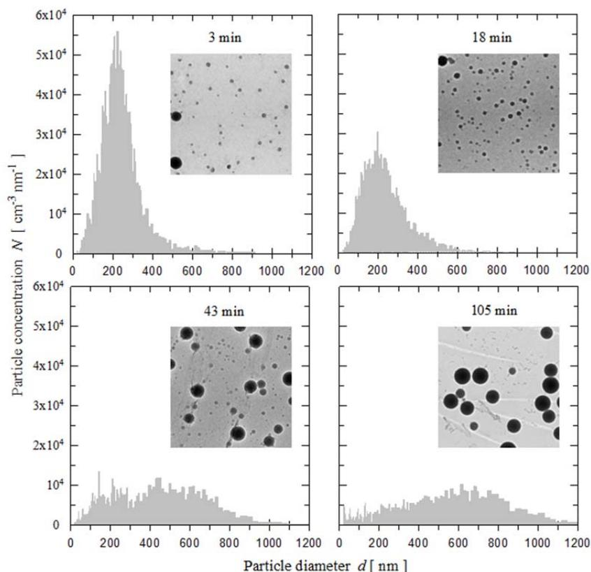
*Figure 7. Particle number size distributions of micelle sample obtained with MANTA's ViewSizer 3000 for different elapsed times as indicated. As in Figure 1, the density function of particle size distribution is shown in terms of histogram. For comparison, TEM images are also shown (courtesy of Nia Bell of UCSD), which support the ViewSizer 3000 data that show a clear trend of increasing average particle size with elapsed time.*
