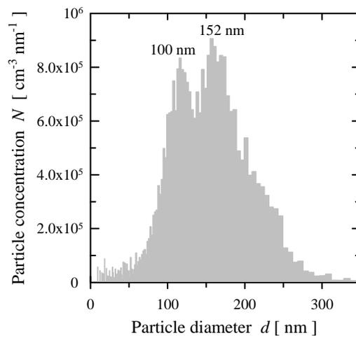
Figure 2. The results were obtained for a sample consisting of the mix of two polystyrene nanosphere size standards, 100 nm and 152 nm. The concentration of particles integrated between 0 and 1,000 nm for this sample was about  $1.0 \times 10^8 \text{ cm}^{-3}$ .
